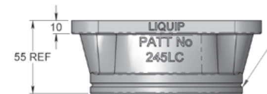
GROOVE AROUND OUTLET IDENTIFIES SLV5-114
