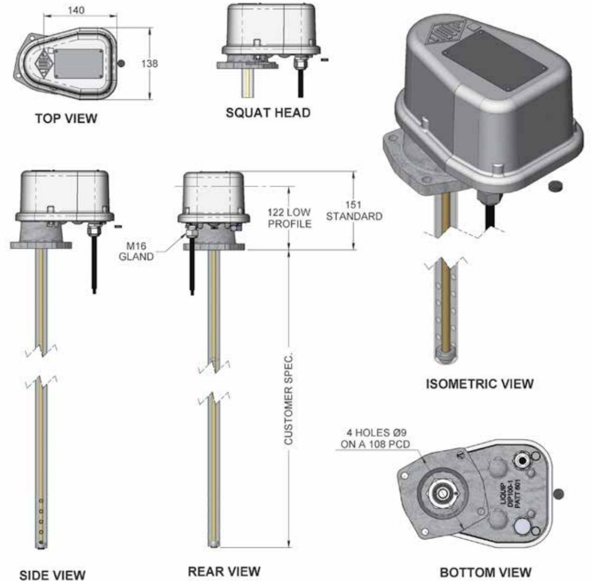
**E.3. DETERMINING THE LENGTH OF SENSOR**
