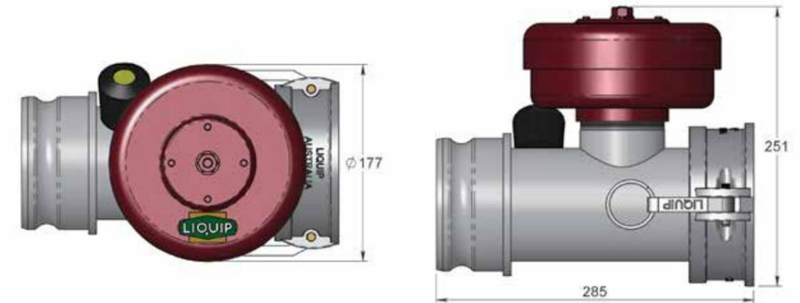
CLOGGING INDICATOR SHOWS BY PERCENTAGE THE INCREASE IN VACUUM PRESSURE DROP UP TO -35mbar (-3.5kPa). PERCENTAGE REMAINS VISIBLE EVEN WHEN VACUUM IS REMOVED. WHEN ELEMENT IS REPLACED, INDICATOR MUST BE MANUALLY RESET BY PRESSING YELLOW BUTTON ON TOP.
