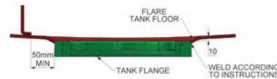
Cut a hole 242-244mm diameter and flare tank shell circumference outwards, for improved drainage and so the tank flange can be welded in easily. Continue flaring until tank flange can fit inside cut out.
