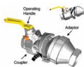
1. Push coupler onto adaptor by first engaging lower jaw of coupler under lip of adaptor and tilting the coupler upward to engage top jaw.
