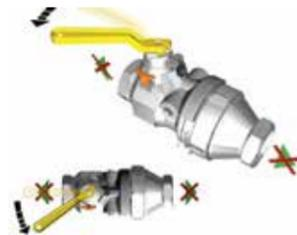
2. Turn handle counter-clockwise until lock engages. Coupler and adaptor are locked together but valve is closed.
