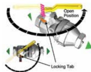
3. Press button on coupler down and turn handle counter-clockwise until it locks. Valve is now open and product will flow.
