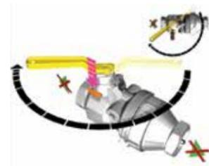
4. To disconnect - press button on coupler and rotate handle clockwise until it locks. Valve is now closed.
