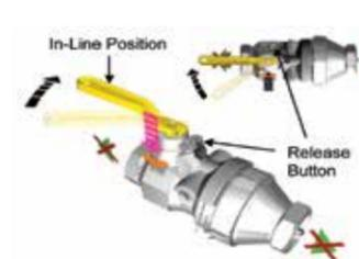
5. Press button on coupler down and turn handle clockwise to the "In-Line" position. Press tab on opposite side of coupler to release the upper jaw and move coupler away.
