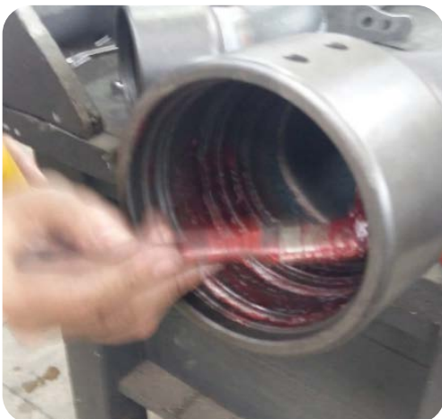
Image 3. Apply the grease with a brush.
