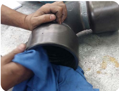
Image 1. Clean the inside of the female body housing.
