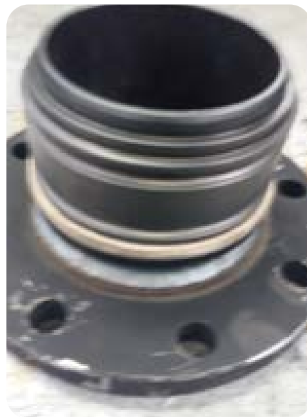
Image 8. Place the dust guard firmly around the male insert.
