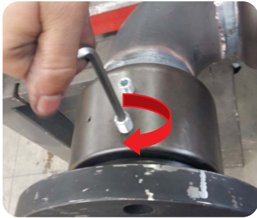
Image 13. Rotate the ball bearing retaining screws clockwise.
