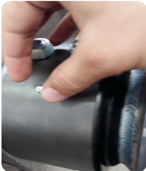
Image 15. Place the grease fitting in the hole.
