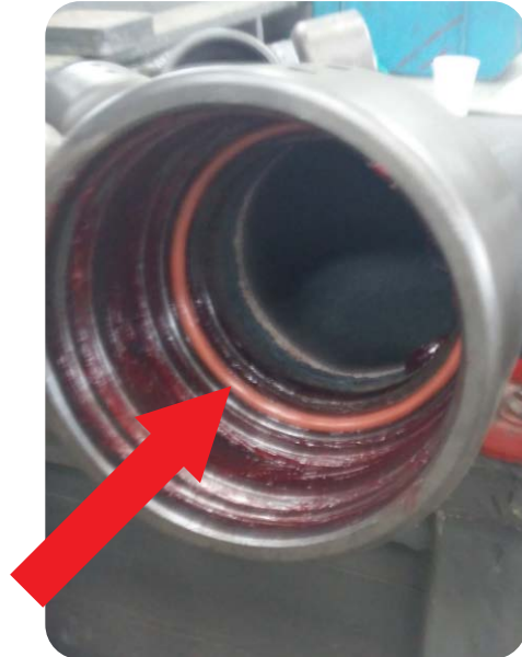
Image 6. The o-ring should be adjusted in the female body.
