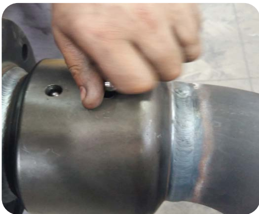
Image 11. Insert the ball bearings into the channel.
