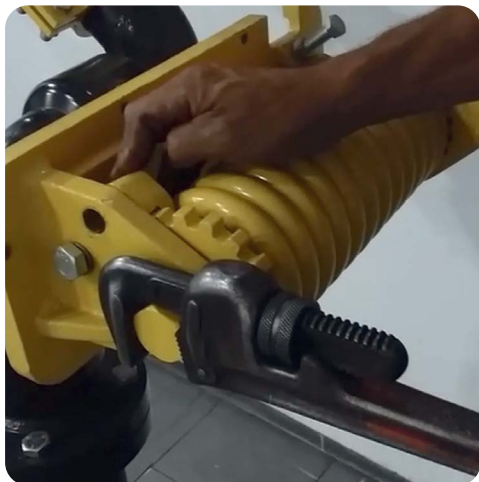
Image 12. Position the latch on the adjustment plate.
