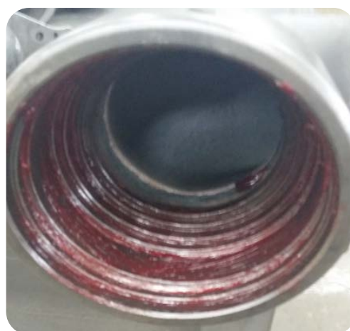
Image 4. Line the entire housing with grease.
