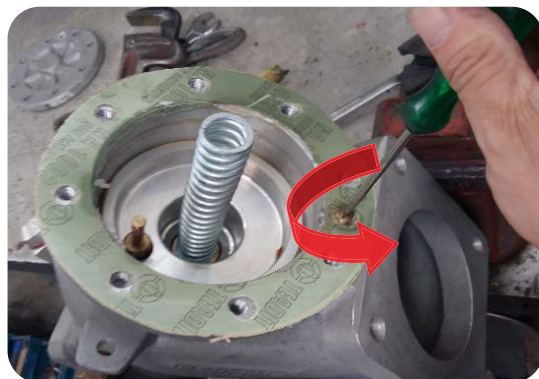
Image 13. Turn counter-clockwise for a faster shut-off.
