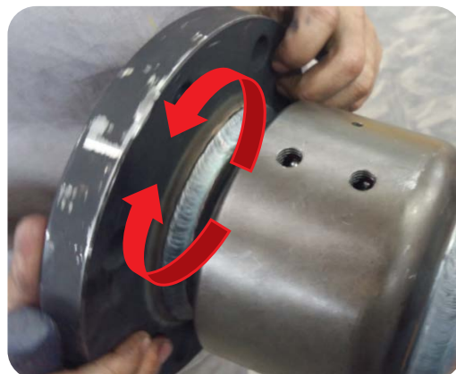
Image 12. Turn clockwise and counterclockwise.
