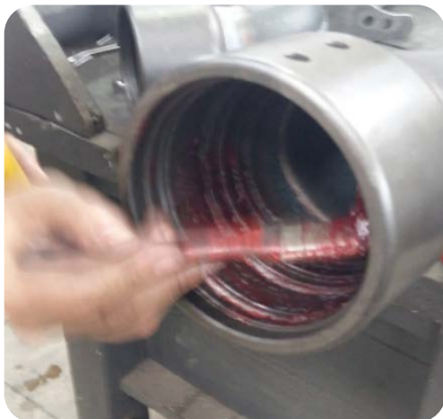
Image 3. Apply the grease with a brush.
