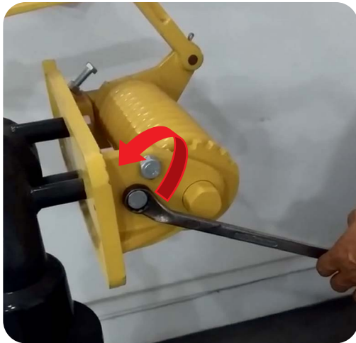
Image 6. Loosen the lower screw.
