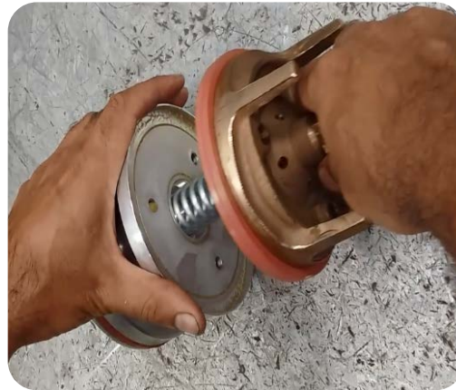
Image 9. Pull the guide, separating it from the piston.
