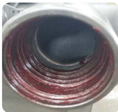
Image 4. Line the entire housing with grease.
