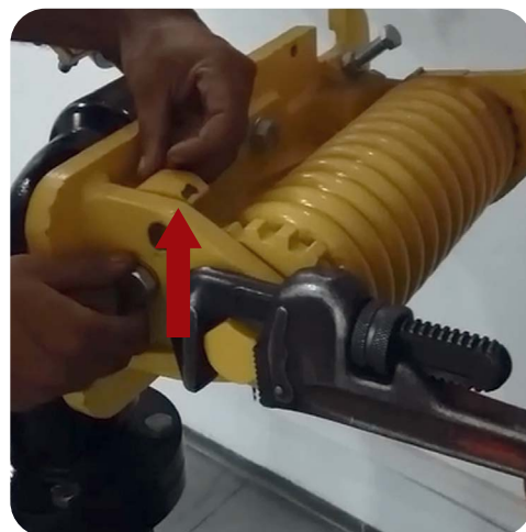
Image 9. Lift the plate latch.
