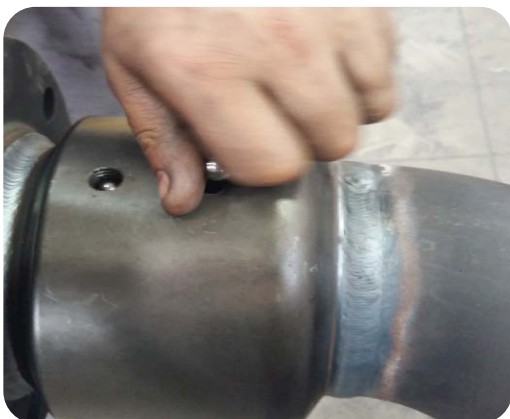
Image 11. Insert the ball bearings into the channel.
