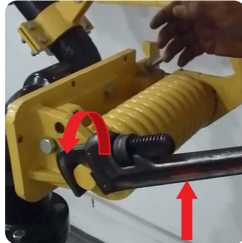
Image 11. For less torque, turn counterclockwise.
