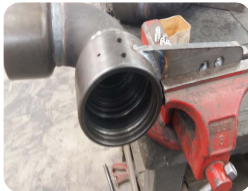
Image 2. Secure the female body to a vise.
