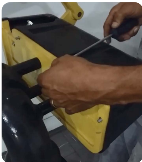
Image 1. Unscrew the protective cover.
