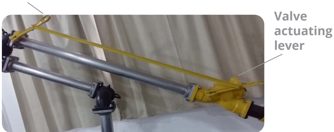
Image 18. Fixed bar on the valve lever up to the remote control lever.
