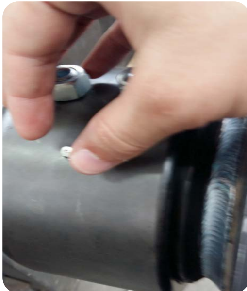
Image 15. Place the grease fitting in the hole.
