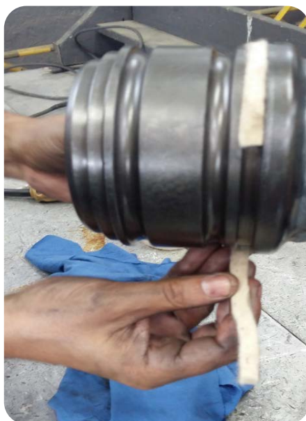
Image 7. Clean the dust guard and male insert .
