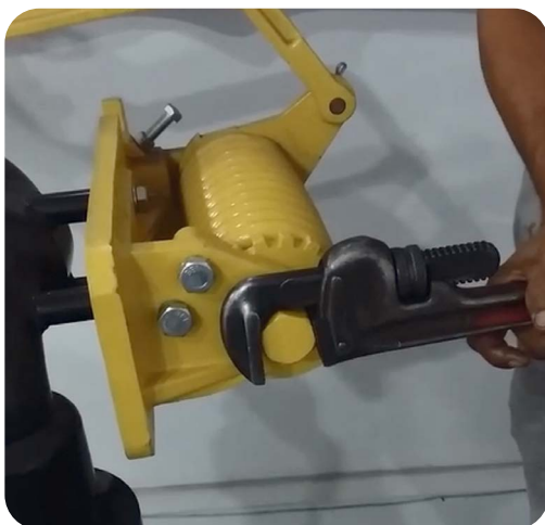
Image 8. Fasten the hex screw of the plate with a pipe wrench.
