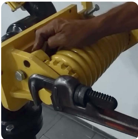
Image 12. Position the latch on the adjustment plate.
