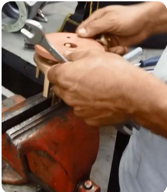
Image 10. Remove the seal to replace it.
