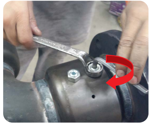
Image 14. Turn the nuts onto the bolts to lock them in place.
