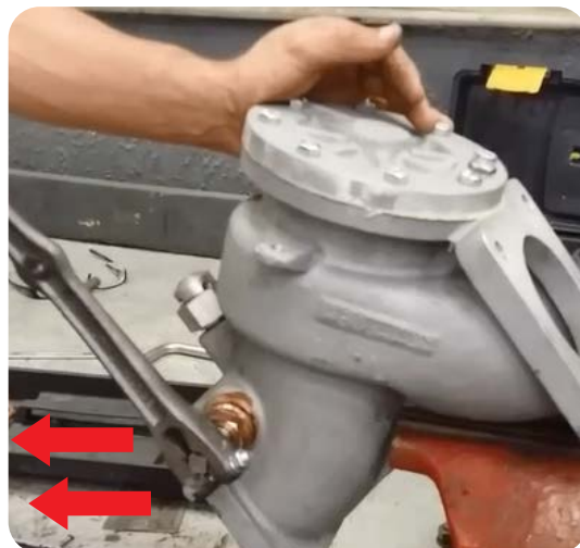
Image 2. When the lever is pulled back, the piston opens the passage for the flow.
