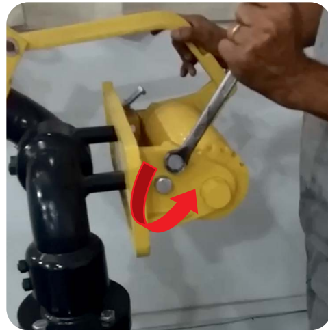
Image 7. Loosen the upper screw.
