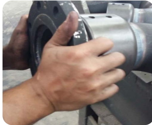
Image 10. Turn the male insert clockwise.
