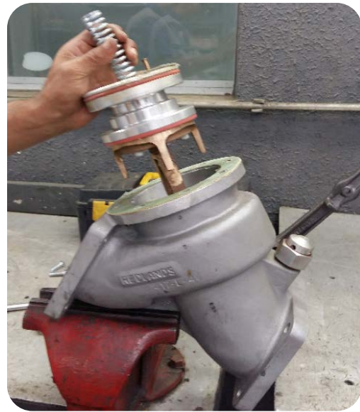
Image 6. Remove the piston subassembly from the valve carefully.
