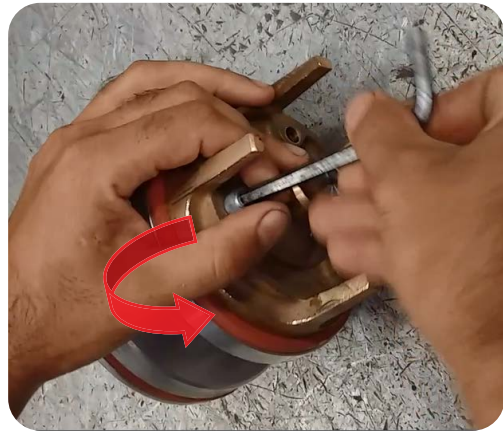
Image 8. Turn the Allen wrench counter-clockwise.
