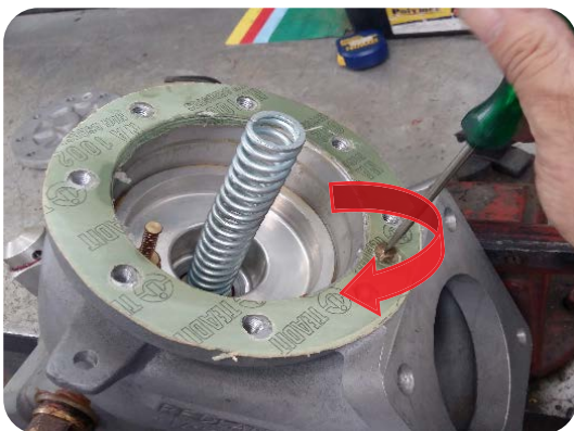
Image 12. Clockwise for a slower shut-off.
