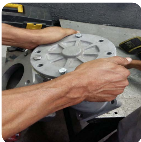
Image 3. Remove all the screws of the valve cover.
