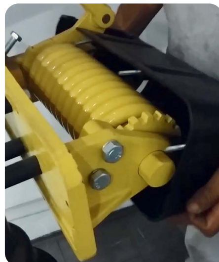
Image 2. Remove the protective cover.
