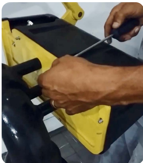
Image 1. Unscrew the protective cover.
