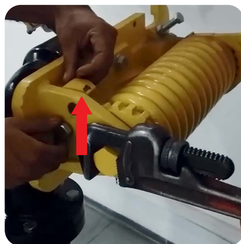
Image 9. Lift the plate latch.
