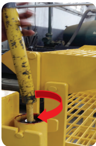
Image 18. Spring pressure by the nut, clockwise.
