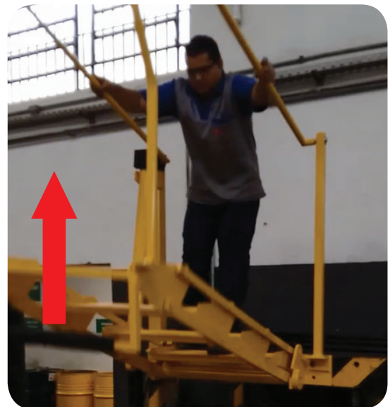
Image 14. Retracting the access gangway.
