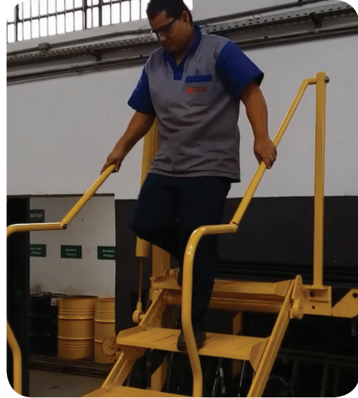
Image 12. Gangway locked by the pedal.
