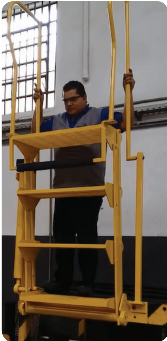
Image 8. Gangway in the upright position.
