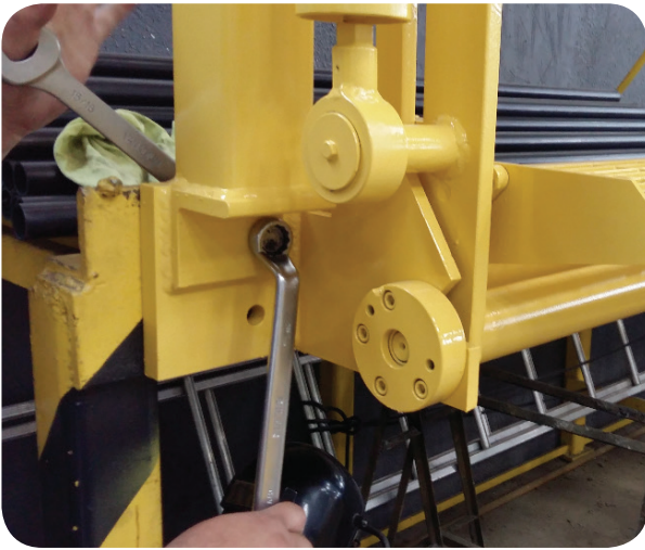
Image 1. Securing the base on the left-hand side.
