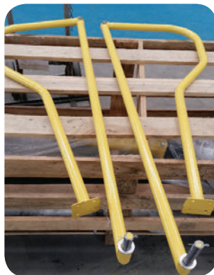
Image 3. Handrail of the access gangway.
