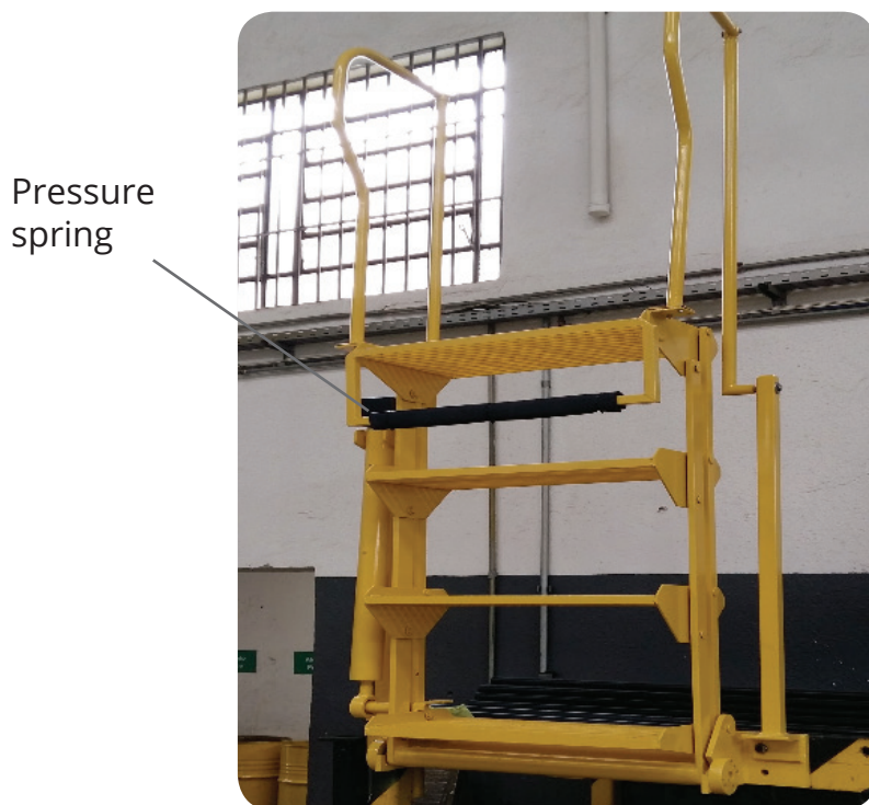
Image 15. Correct position for maintenance on the spring.
