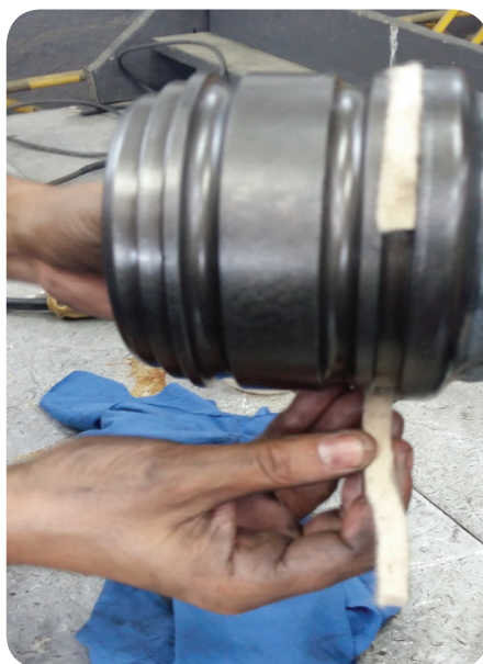
Image 7. Clean the dust guard and male insert.
