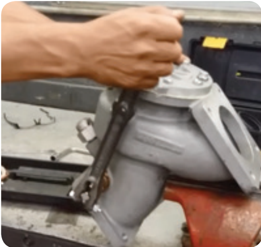
Image 1. Operate the valve using the lever to vent the air trapped in the cylinder.
