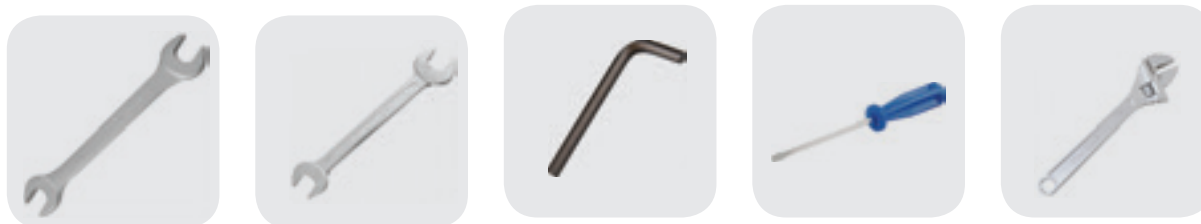
Image 1. Tools used for maintenance and adjustment of the 417 valve.
