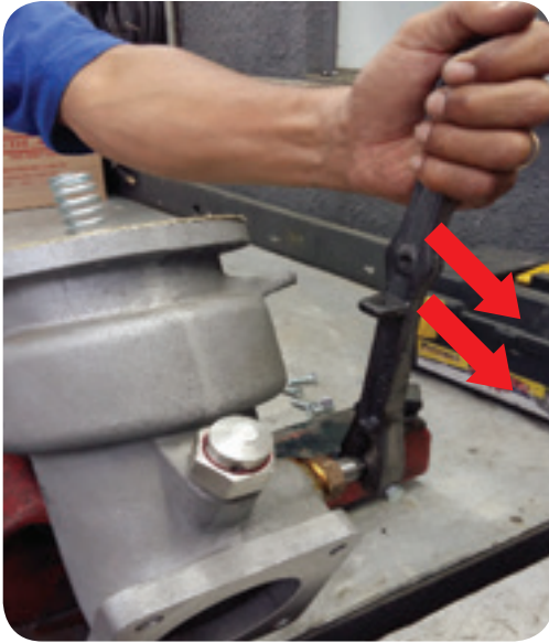
Image 5. Move the lever forward and release the piston assembly.
