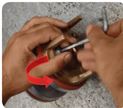
Image 8. Turn the Allen wrench counter-clockwise.
