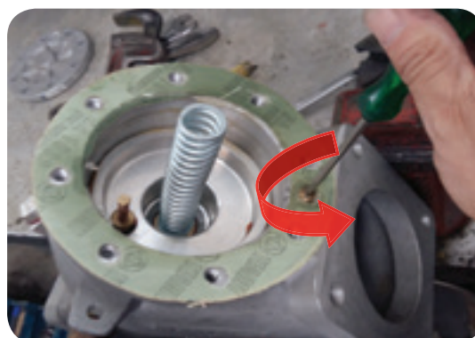
Image 13. Turn counter-clockwise for a faster shut-off.
