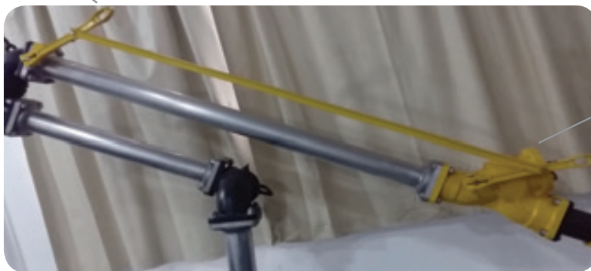
Image 18. Fixed bar on the valve lever up to the remote control lever.
