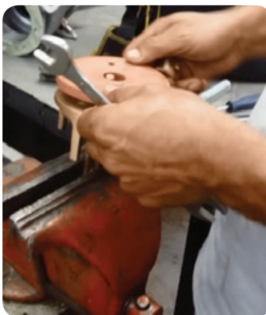
Image 10. Remove the seal to replace it.
